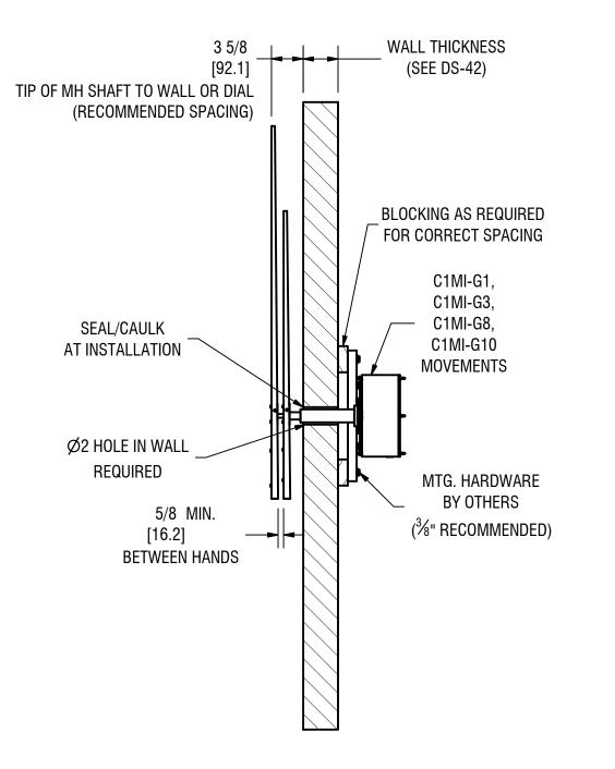
REFER TO DS-42 FOR COMPLETE MOVEMENT SPECIFICATIONS G12MI MOVEMENT INSTALLATION REFER TO DS-533 ALL DIMENSIONS: INCHES [MILLIMETERS]
