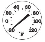
10) IF POINTER WAS PROVIDED SEPARATELY, INSTALL POINTER ONTO DIAL POINTING TO LOWEST READING ON DIAL (-20°F SHOWN)
