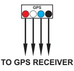
Connect GPS Receiver to "GPS" terminals, matching wire colors to colors shown on wiring diagram on inside cover of terminal compartment
