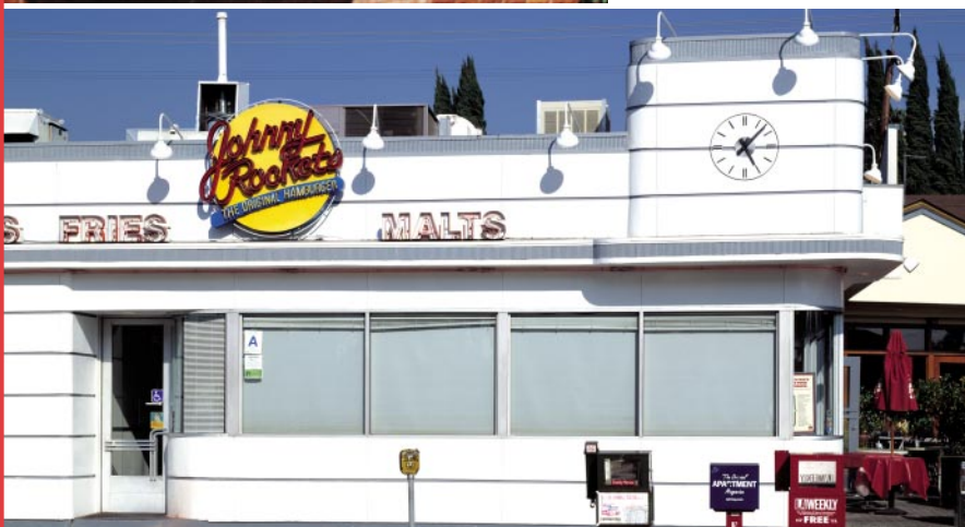
PHOTO TOP LEFT: Outdoor Style 1100 Silhouette Clock 60" in diameter, with type MS-A hands, type A dial markings, and special trim ring to have a custom green painted finish, color to be selected by architect. Rear access movement to accommodate a 1 3/4" thick wall. Type 99B remote reset control to be located in building electrical room.
